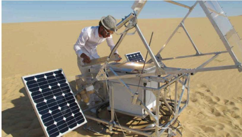
Glass is printed in the Sahara desert with sand “ink” and a solar powered 3D printer.
